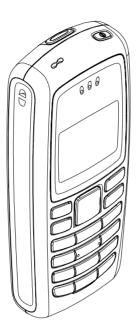
The NAM-2 is a dual band transceiver unit designed for the GSM900 (including EGSM) and GSM1800 networks. It is both GSM900 phase 2 power class 4 transceiver (2W) and GSM1800 power class 1 (1W) transceiver.
